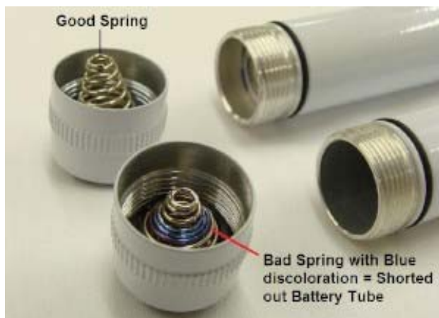
Picture of a good and shorted out battery tube spring.
