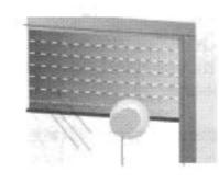
Stick the suction cap of the brightness sensor to the inside of the window pane at the desired shade position of the roller shutter.
